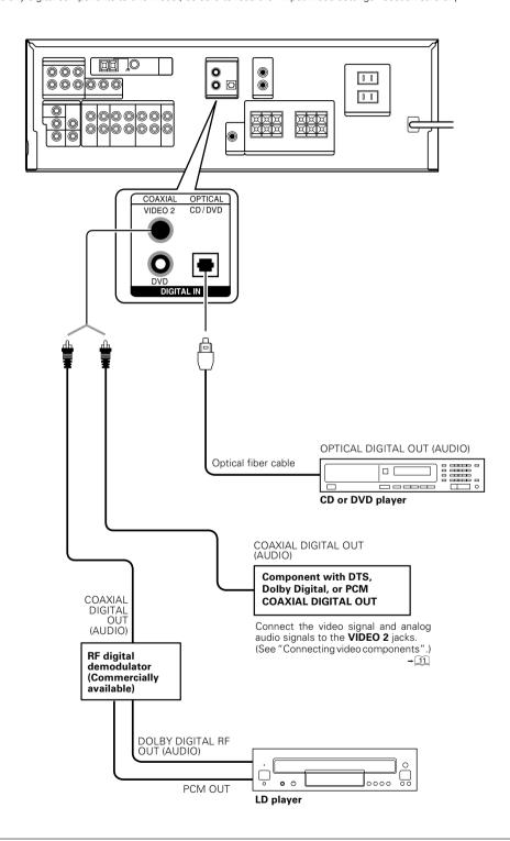
To connect an LD player with a DIGITAL RF OUT, connect the LD player to the RF digital demodulator (Commercially available). Next, connect the DIGITAL OUT jacks of the demodulator to the DIGITAL IN jacks of this model. Connect the video signal and analog audio signals to the VIDEO 2 jacks. (See "Connecting video components".)
